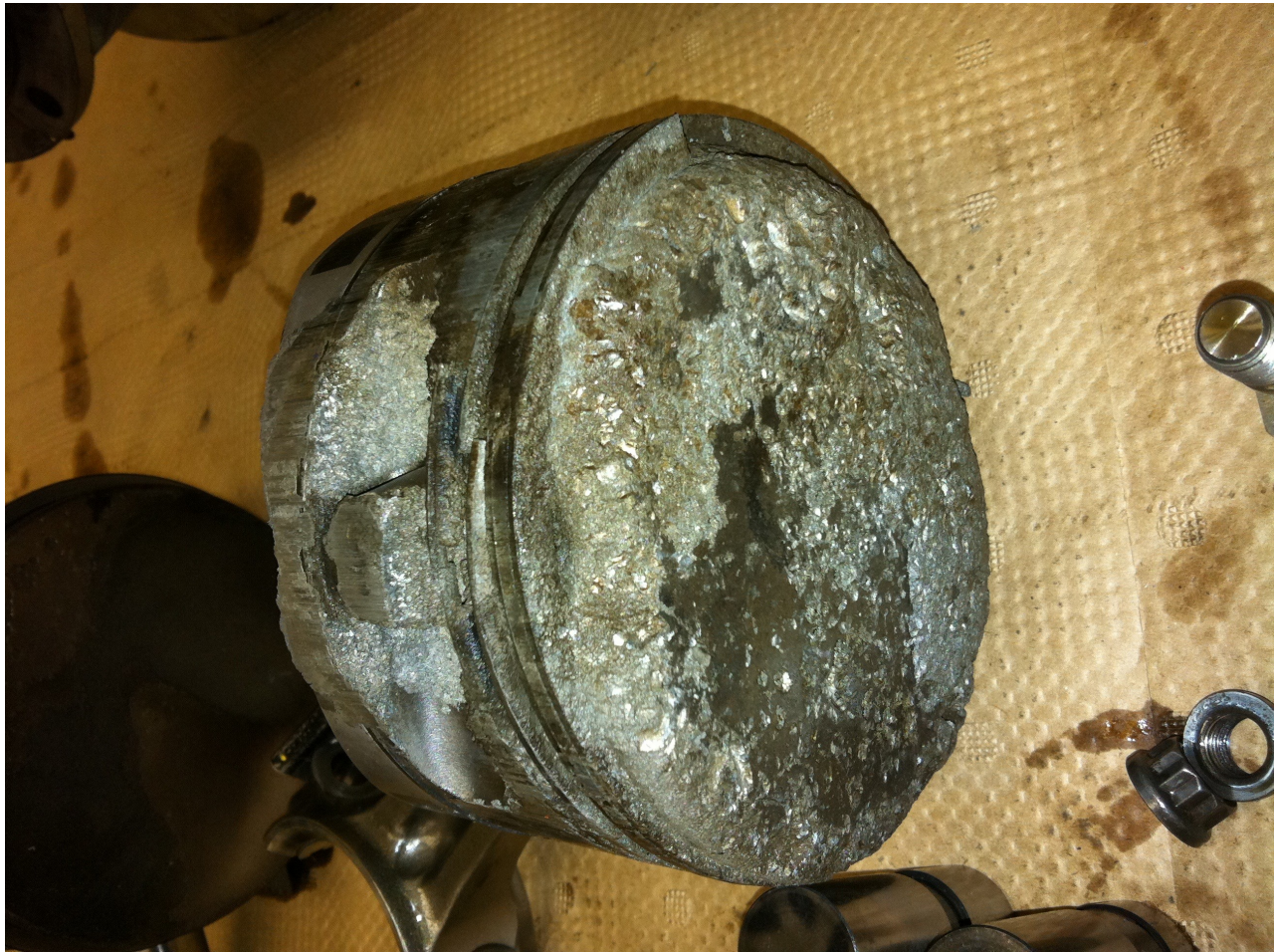
Figure 2-9. An aircraft piston showing damage that occurred in just minutes as a result of detonation and overheating.
