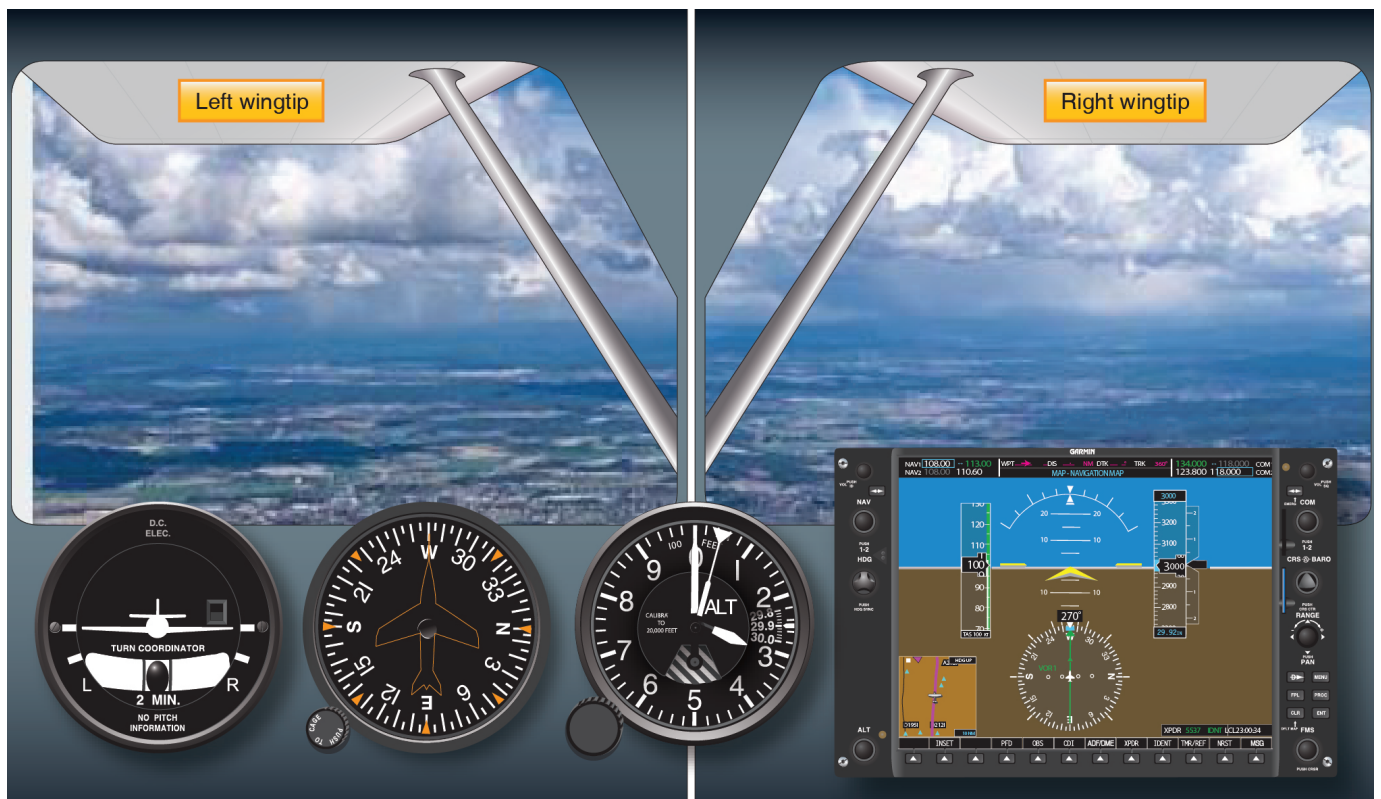
Figure 3-7. Wingtip reference for straight-and-level flight.
