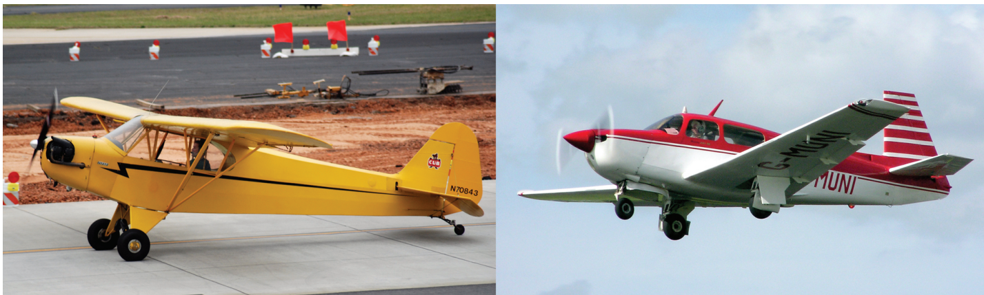
Figure 14-1. The Piper Super Cub on the left is a popular tailwheel airplane. The airplane on the right is a Mooney M20, which is a nose-wheel (tricycle gear) airplane.
