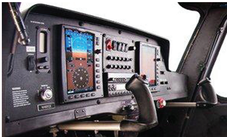
Figure 17-11. Stoke flight control with conventional engine controls.
