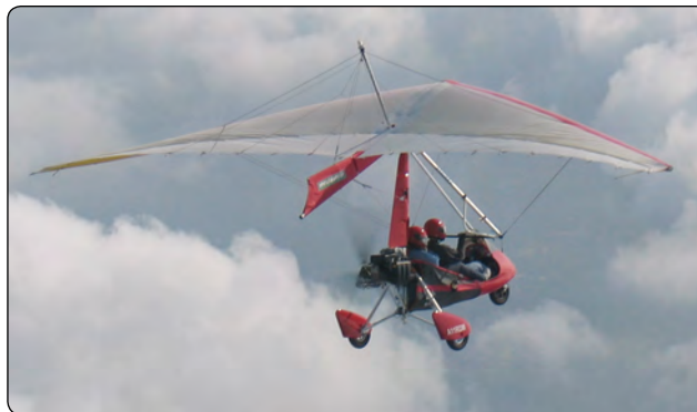
Figure 3-9. Weight-shift control aircraft use the shifting of weight for control.
