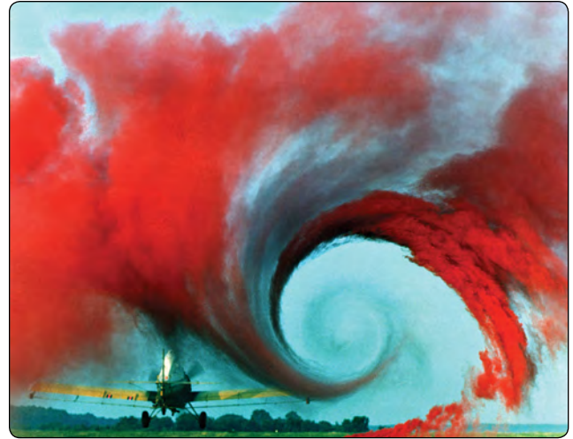
Figure 5-9. Wingtip vortex from a crop duster.
