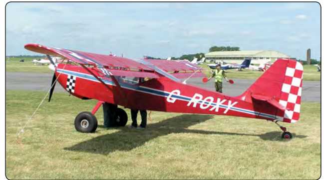
Figure 6-9. Flaperons on a Skystar Kitfox MK 7.
