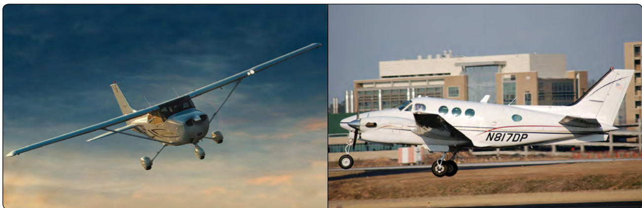
Figure 7-39. Fixed (left) and retractable (right) gear airplanes.
