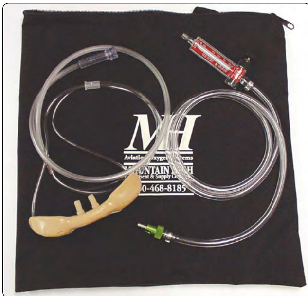
Figure 7-44. Cannula with green flow detector.
