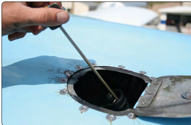
Figure 7-18. Always check the engine oil level during the preflight inspection.
