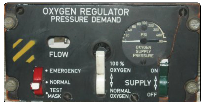
Figure 7-43. Oxygen system regulator.
