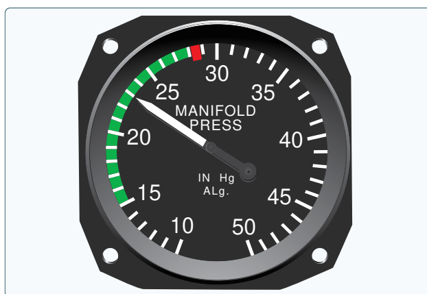
Figure 7-9. Engine power output is indicated on the manifold pressure gauge.
