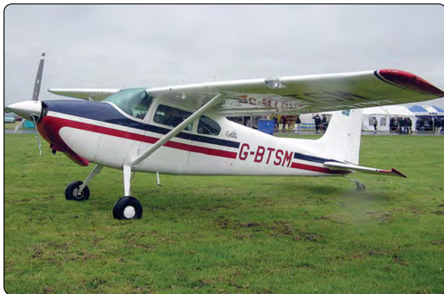
Figure 7-38. Tailwheel landing gear.
