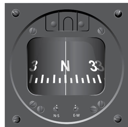
Figure 8-32. A magnetic compass. The vertical line is called the lubber line.
