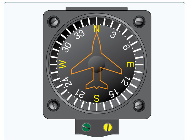
Figure 8-38. Vertical card magnetic compass.
